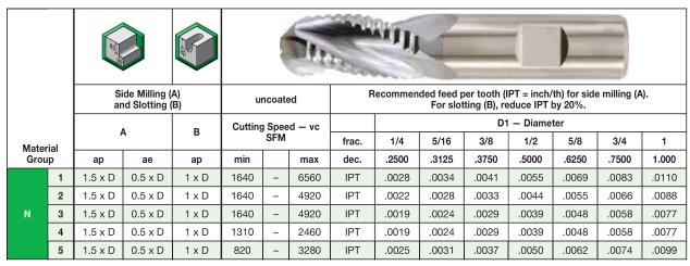
NOTE: For cutting aluminum with high silicon, coating is recommended.
